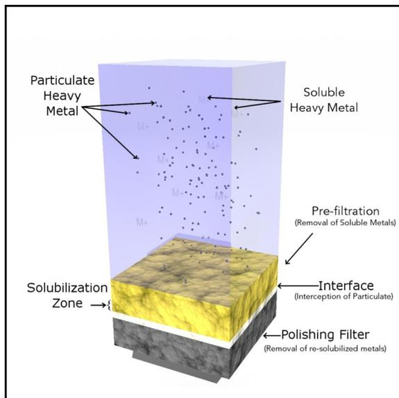
Fig. 2. Diagram showing the system for removing heavy metal solutions that contain soluble and partially insoluble species.
