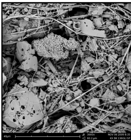
Fig 3. SEM of the surface of one of the two layers showing the immobilized adsorbents and tight pore structure.
