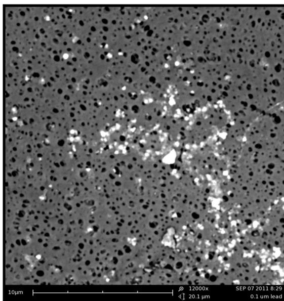
Fig. 1. SEM of particulate lead filtered through a 0.1 micron syringe filter to show size. Lead was precipitated according to NSF/ANSI 53.
