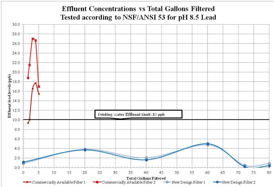
Fig. 4. Testing results when tested to NSF/ANSI 53 for pH 8.5 lead.
