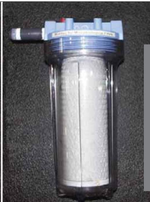
The filter 1 system incorporated two housings—one containing a pleated prefilter (far left) to remove coarse particulate matter and a second containing an extruded activated carbon filter (middle). The photo on the right shows the second filter in the housing.
